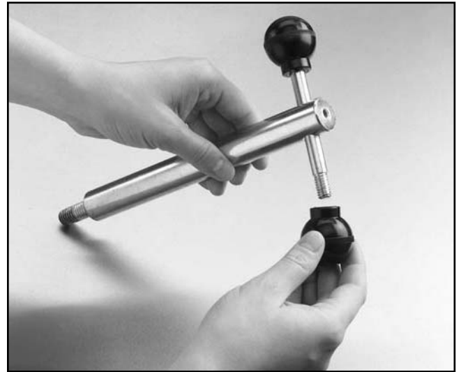
Figure 10. Thread round knobs onto bar.
